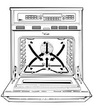
Because food is heated faster in a convection oven when using the convection modes, many types of food can be cooked at lower temperatures than those suggested for regular ovens. Do remember that recipe books often give times and temperatures for cooking in regular ovens. Convection ovens make it possible to reduce the temperature by 25°F.
